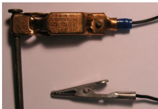
The larger clip is the positive (anode) side and will not come in contact with the solution.
